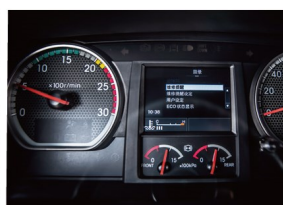
Multifunctional 4-inches liquid crystal display which pursues "easily watching and understanding"
